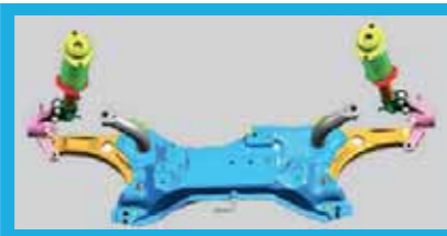
Frame type front suspension system for smoother drives
