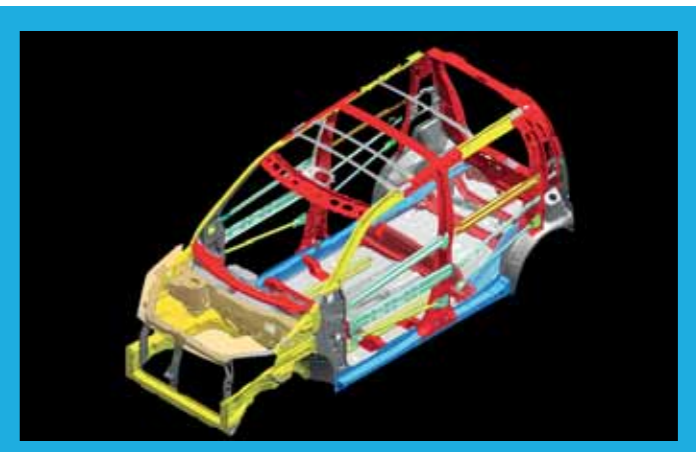
Energy absorbing body structure for safer drives
