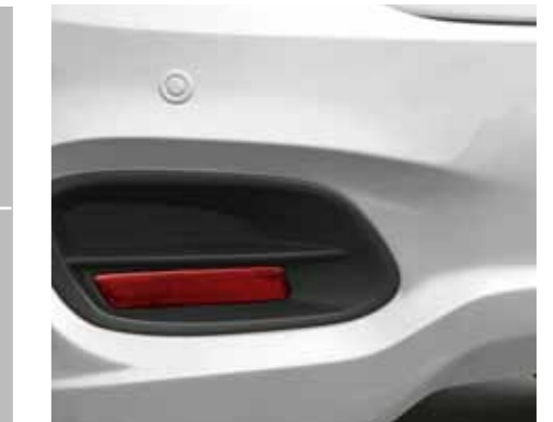
Rear Parking Sensors
